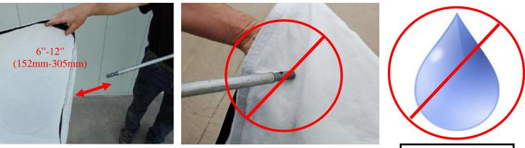
LIGHTLY CLEAN WITH COMPRESSED AIR ONLY, FROM THE OUTSIDE IN. KEEP THE NOZZLE 6-12 INCHES FROM FABRIC
